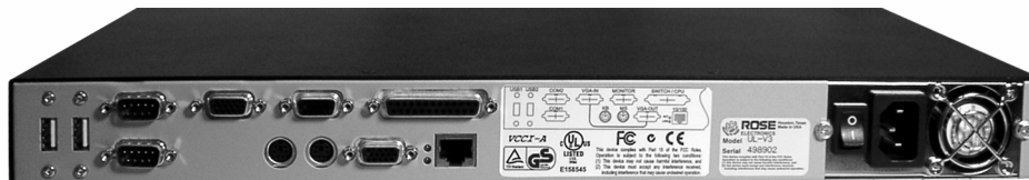
Figure 2 External connections on the back panel
